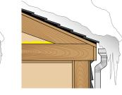
When snow and ice melt, trapped water can infiltrate to damage the roof deck and building interior.
